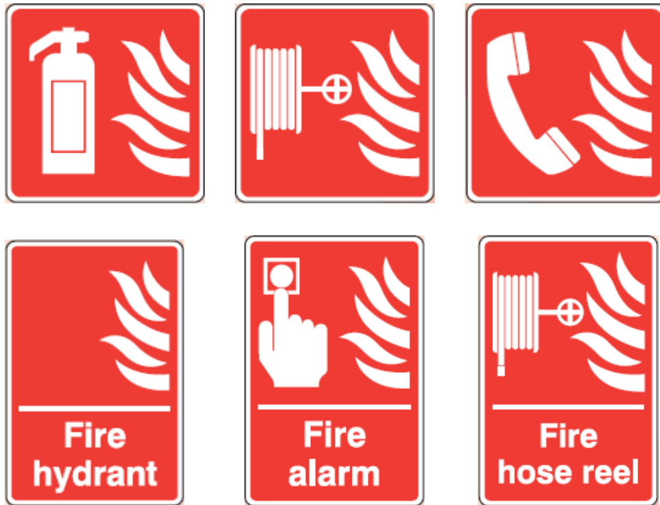
Figure 17 - Fire point equipment signs
